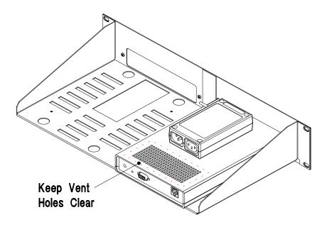
Figure 3-12: LanProbe Installed in the Rack Support Shelf
